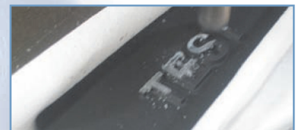
Step 6: Raised Text – sand or mill paint to expose the areas to be illuminated
