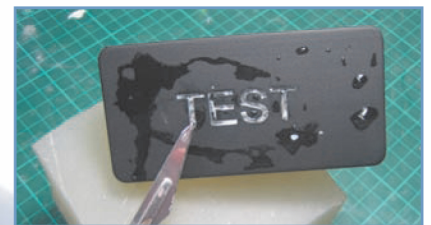
Step 6: Recessed Text – use scalpel or WaterJet
