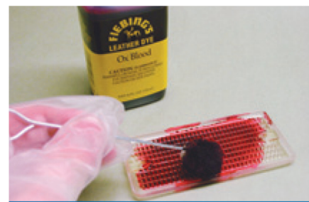
Figure 2: Apply aniline dye Aniline dye is applied to the model by brushing (shown), or dipping
