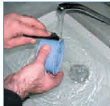
Figure 2. Wet-sanding. Wet-sand the model with 320-grid sandpaper.
