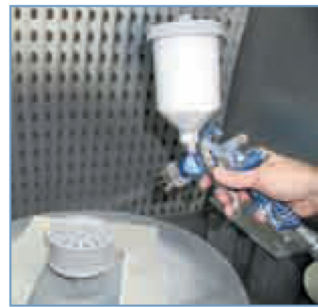
Figure 6. Apply Primer Paint.
