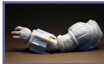
1a. Cleaned and dried model with support material removed.
