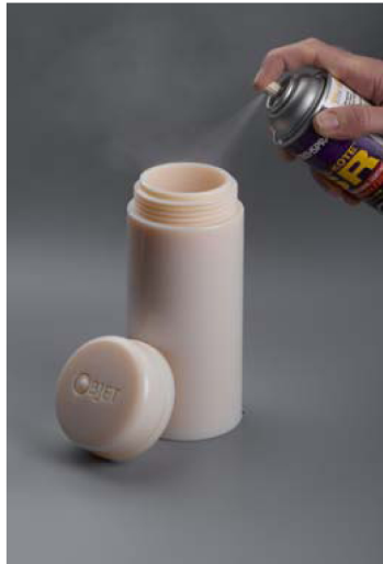
Figure 3. Coating the inner surface of the bottle
