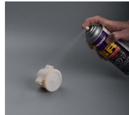
Figure 2. Applying chemical resistance spray on assembled parts
